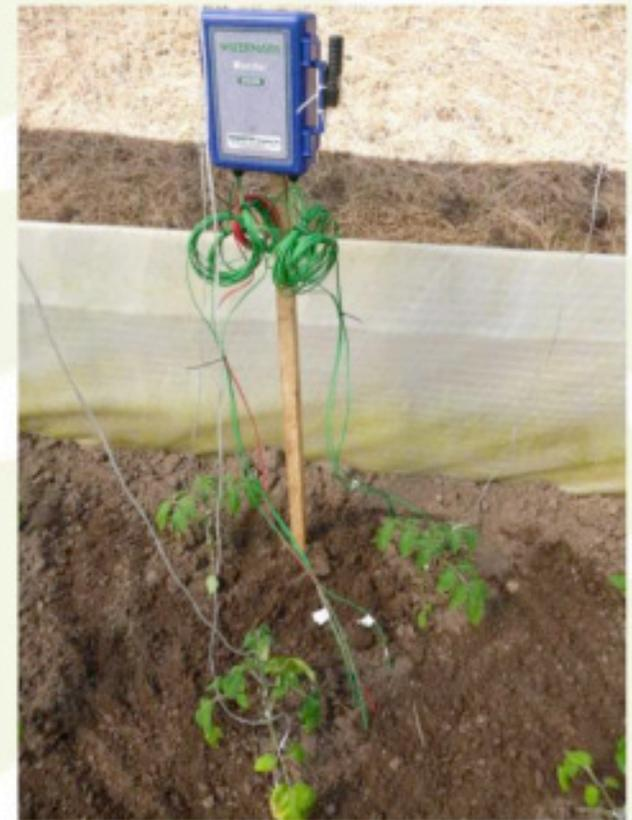
Installation of WaterMark sensors, recording with a datalogger on each plot.
