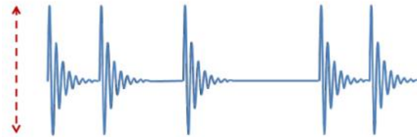
Figure 2: An example of a short section of the Hydropath Signal. The red arrow indicates the “peak-to-peak voltage”. (Rodrigues, 2012).
